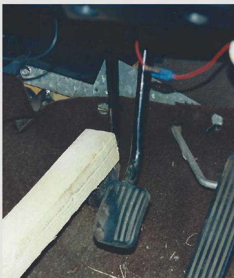
Above: Wedging a clutch pedal down when a car is stored will prevent the plate from becoming rusted on to the flywheel.
